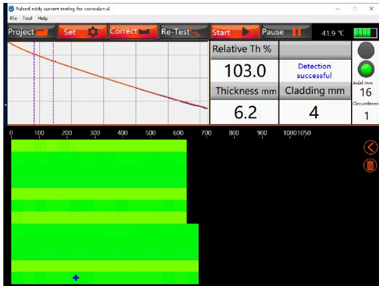
Figure 4-10 C-scan image of corrosion thickness measurement
