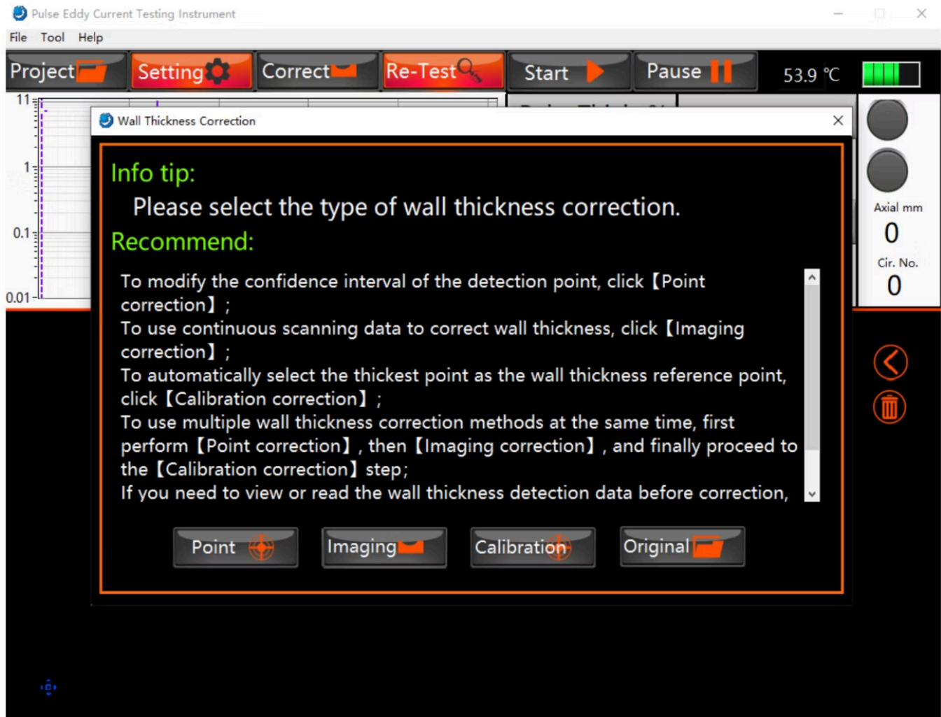
Figure 5-6 Wall thickness correction
