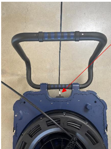
Fig. 112: Correct fit of the reel
