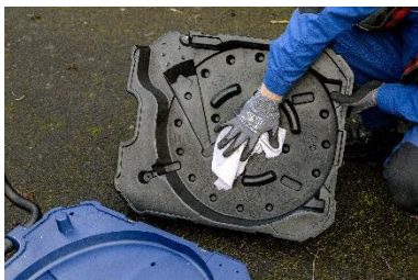
Fig. 107: The lower shell can be cleaned with a damp cloth.
