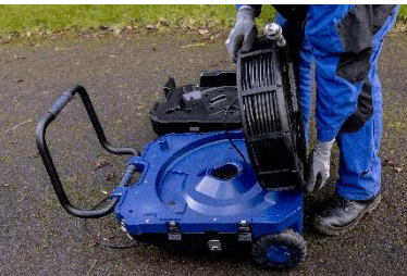
Fig. 110: Place the reel in the reel holder
