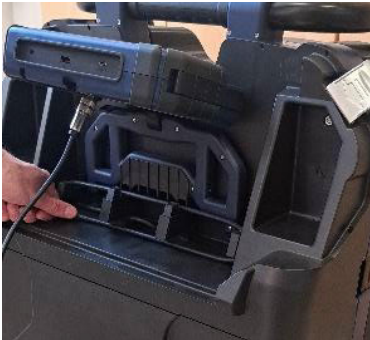
Fig. 114: Wrap the monitor cable around the cable domes
