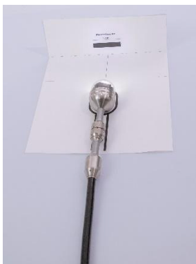
Fig. 82: Calibration with calibration template
