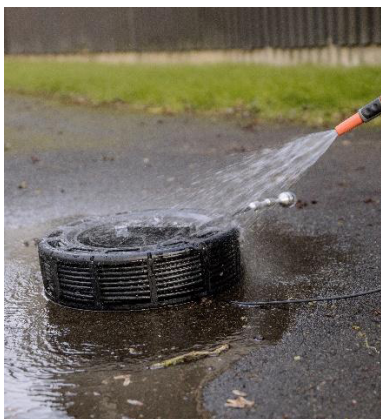
Fig. 106: Hosing off the reel and rod
