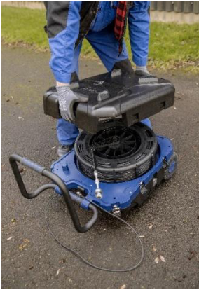
Fig. 19: Place the lower tray on top
