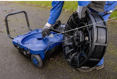
Fig. 109: Pull the connection cable through the opening of the reel holder
