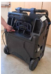
Fig. 43: Roll up the connection cable before pushing the monitor back in.
