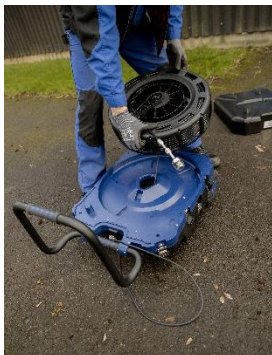
Fig. 104: Pull the reel out of the reel holder
