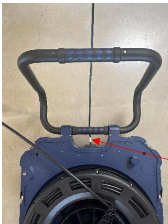
Fig. 18: Correct fit of the reel
