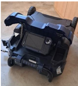
Fig. 46: Wöhler VIS 750 HD inspection camera in horizontal position with glare shield
