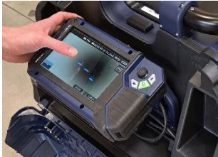
Fig. 85: Set the start and end point of the measuring section.
