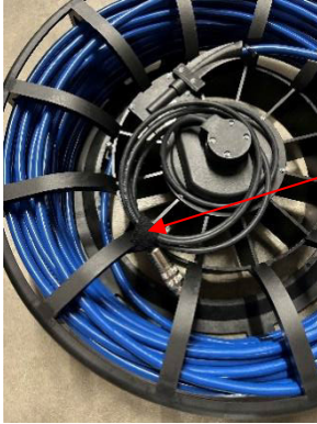
Fig. 14: Velcro on the monitor cable
