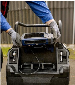
Fig. 100: Pull up the monitor to remove it and the stand from the holder
