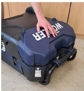
Fig. 21: The front flap should engage clearly when inserted
