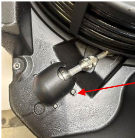
Fig. 26: Attaching the transport lock
