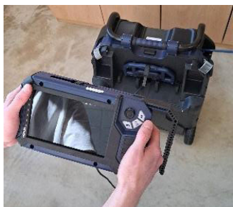
Fig. 40: Monitor pulled out of the trolley holder
