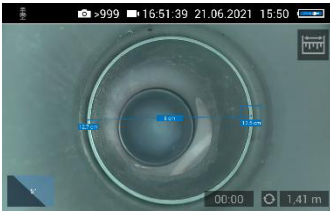
Fig. 78: Display of the distance between two measuring points
