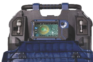
Fig. 39: Transport position of the monitor
