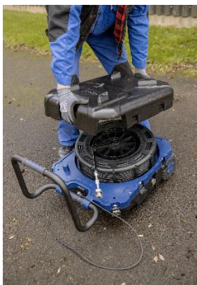
Fig. 103: Remove lower shell
