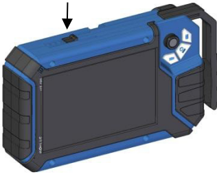
Fig. 45: Push button for pulling out the handle marked with an arrow
