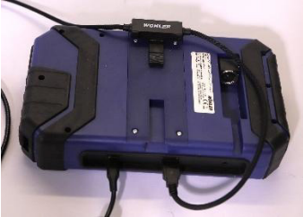
Fig. 28: VE probe adapter on the monitor
