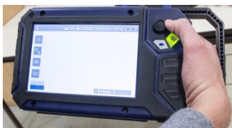
Fig. 44: When the handle is extended, the monitor can be held and operated with one hand.
