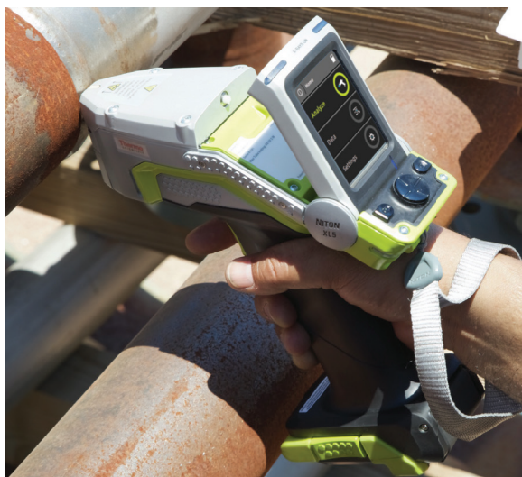
The Thermo Scientific Niton XL5 in use, analyzing parts utilized in metal fabrication and manufacturing processes.
