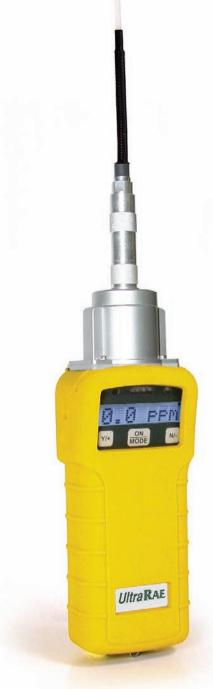
UltraRAE is a quick spot-check monitor, typically used by occupational health, safety and environmental personnel. The combination filter tube and PID removes the disadvantages associated with colorimetric tubes and gas chromatographs. Applications include tank entry pre-screening during refinery and plant maintenance, hazardous material response, marine spill response and refinery down-stream monitoring.
