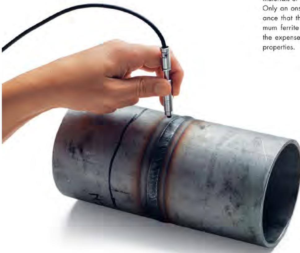
Measurement of the ferrite content of a weld seam
