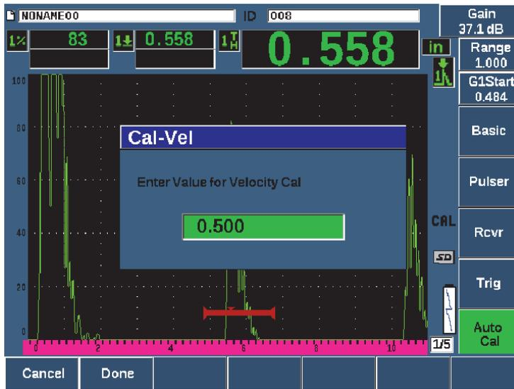
Figure 9-4 Entering the Velocity Cal thickness value
