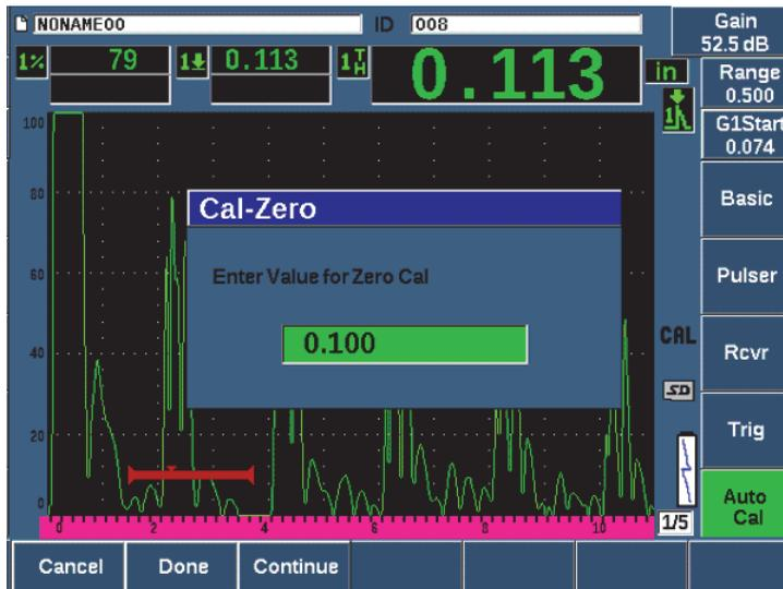
Figure 9-7 Entering the Zero Cal thickness value
