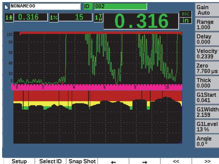
Figure 11-47 B-scan display in the Data Logger
