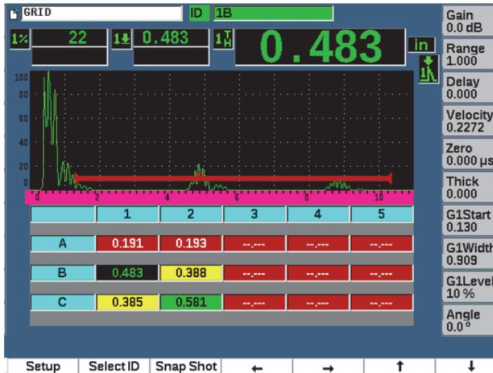
Figure 10-26 Grid controls in Contents screen
