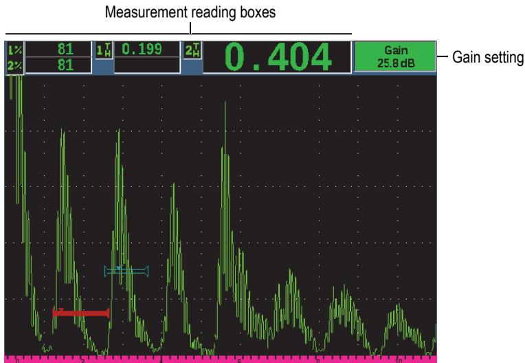
Figure 4-2 Software display elements in full screen mode
