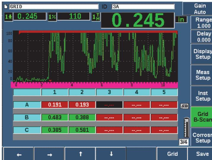
Figure 11-37 Corrosion Module grid view
