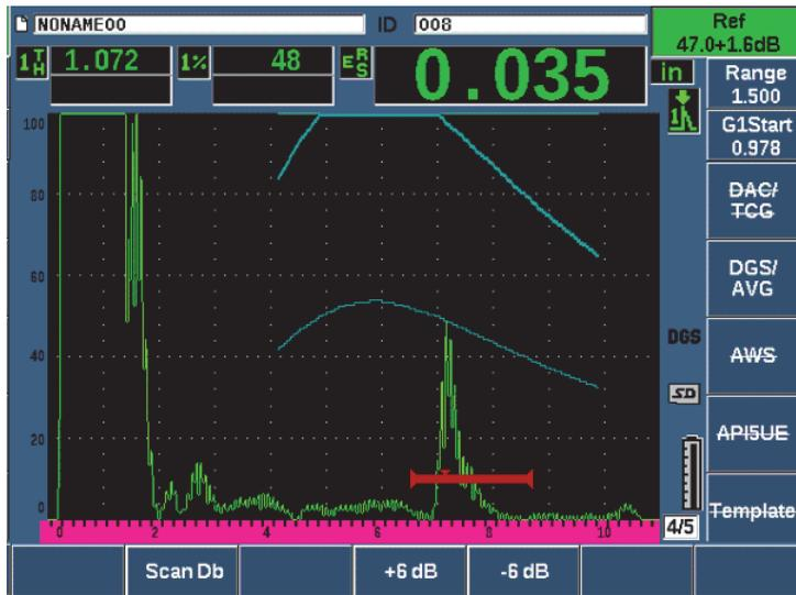
Figure 11-17 Gain curve adjusted DGS
