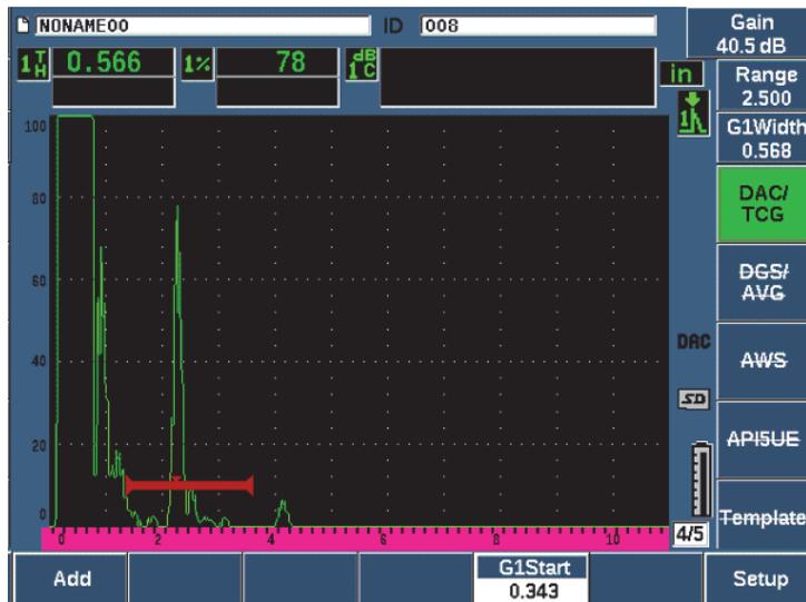
Figure 11-3 First DAC setup step
