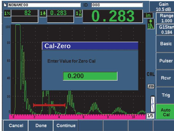
**Figure 9-2 Entering the Zero Cal thickness value**
