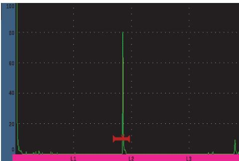
**Leg grid:** displaying vertical lines representing angle beam inspection legs. This mode displays up to 4 divisions, labeled **L1** to **L4**, which represent each half-skip distance of a test piece during an angle beam inspection. The spacing and number of divisions displayed depends on the **Basic > Range**, **Basic > Delay**, and **Trig > Thick** (material thickness) parameters.
