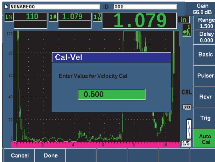
Figure 9-13 Entering the Velocity Cal thickness value
