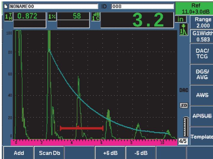
**Figure 11-9 Standard DAC with 3 dB scanning gain**
