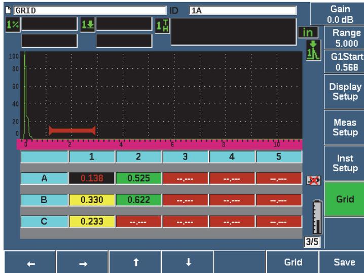
Figure 10-25 Grid controls in the live screen
