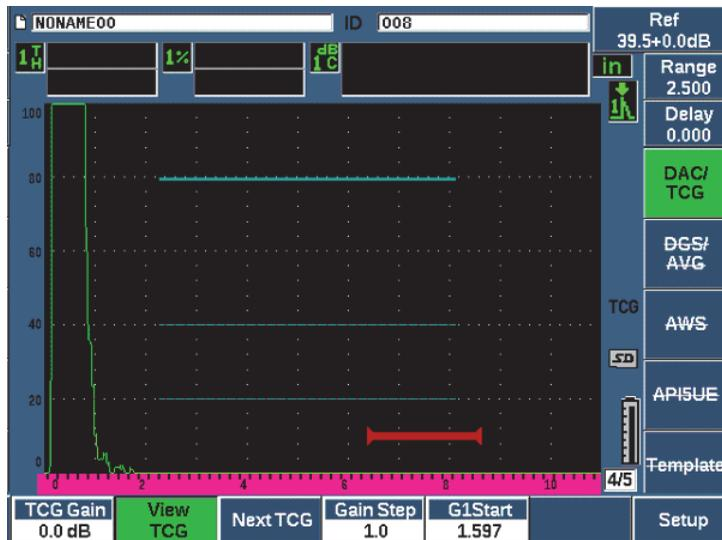
Figure 11-7 Completed DAC curves in TCG view mode
