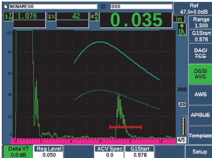
Figure 11-16 DGS/AVG curves on screen
