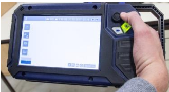
Fig. 15: With the handle pulled out it is possible to hold and operate the monitor with one hand.
