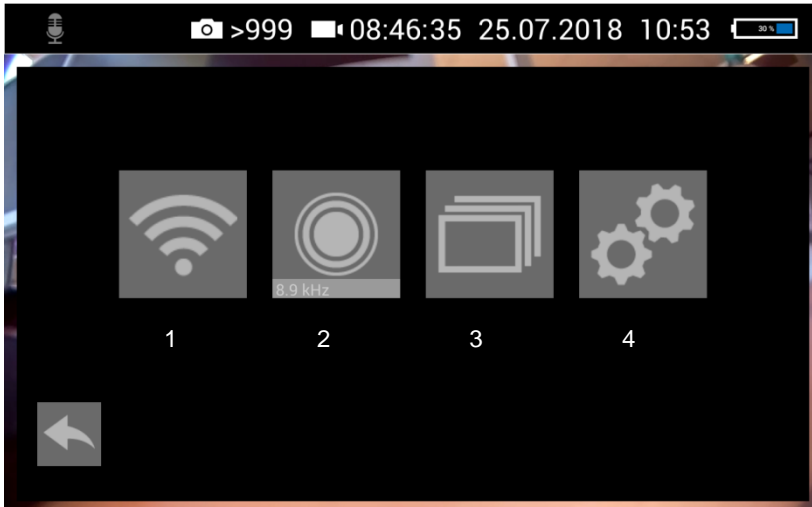
Fig. 32: System menu with submenus WLAN (1), Locator detection (2), Image and video gallery (3) and settings (4)
