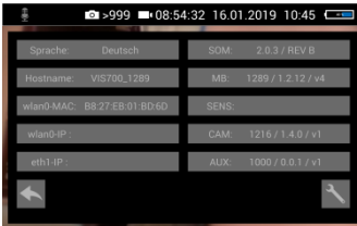
Fig. 54: Info menu with SOM (Firmware of the camera) and CAM (Version of the camera head)
