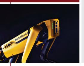
Spot's built-in stereo cameras provide depth information to produce 3D point clouds, enabling the robot to map its surroundings and avoid obstacles. These cameras are primarily for the robot's own navigation but also provide the user with a live monochrome video feed that can be streamed through the control tablet or over the API. For high-definition, color images or increased range in 3D mapping, consider adding a Spot CAM or LIDAR to the system.
