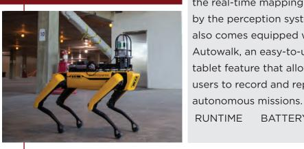
Spot autonomously navigates over or around obstacles in its path using the real-time mapping conducted by the perception system. Spot also comes equipped with Autowalk, an easy-to-use tablet feature that allows users to record and replay
