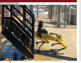
Spot's legs keep the robot stable while it quickly navigates stairs and difficult terrain. Register additional payload weight and watch as the system automatically adapts to keep the robot moving smoothly.
