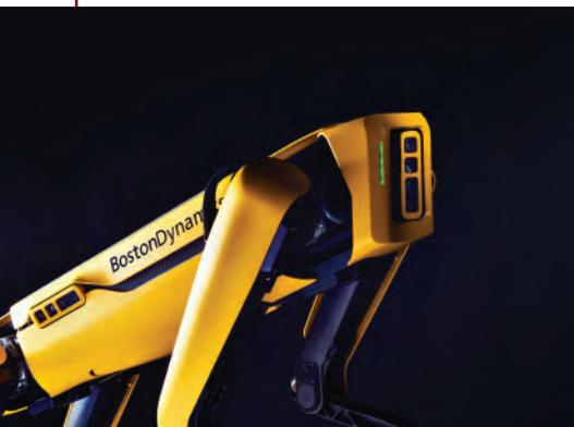
Spot's built-in stereo cameras provide depth information to produce 3D point clouds, enabling the robot to map its surroundings and avoid obstacles. These cameras are primarily for the robot's own navigation but also provide the user with a live monochrome video feed that can be streamed through the control tablet or over the API. For high-definition, color images or increased range in 3D mapping, consider adding a Spot CAM or LIDAR to the system.
